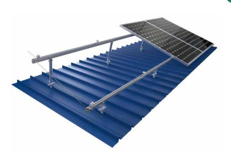
Sunpal adjustable tilt system is used for metal roof concrete roof, you can fixed or adjustable angle as 10-15deg, 15-30deg and 30-60deg options to maximize energy production. All Products pre-assembled before shipment, to make the installation easy and quickly. Unique design of inner and outer tube with adjustable Joint, made structure stronger, different from the same type products on the market today, and widely compatible with standing seam clamp.
